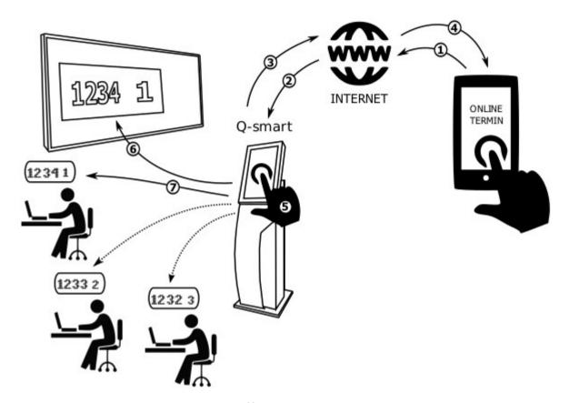
Q-smart queue management system is offered with integral Web server and appointment Webpage. Using the ticket dispenser connected to the Internet, the customer connects through the URL you have specified (1+2).
