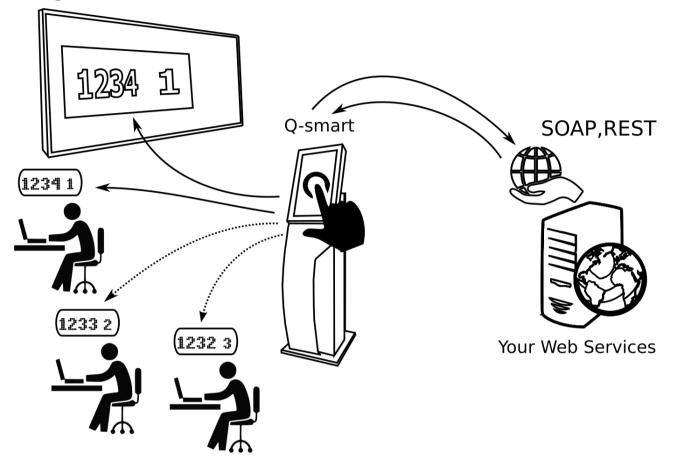
Q-smart queue management system is designed through an architecture that communicates with the external world. The system calls to your web services all the information needed for your customer relations management operations like when a ticket is taken, when a customer with an appointment is called, when a survey form is entered, when a ticket is called, when the card reader reads a private customer or when a new appointment is made.
